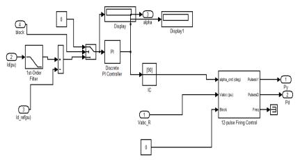
Fig 3. Rectifier control with PI.
