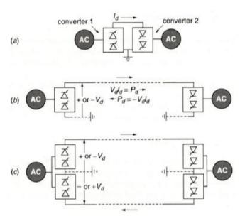
Fig 1. Schematic diagram of an HVDC back to back system
