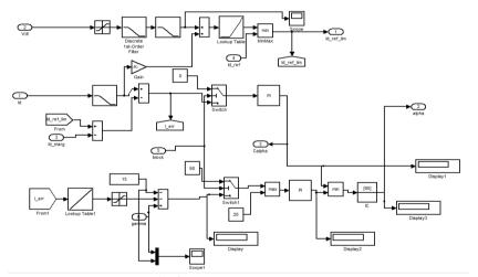
Fig 4. Inverter control with PI.
