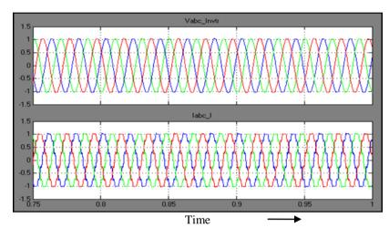
Fig 7. Inverter side AC Voltage ad AC Current
