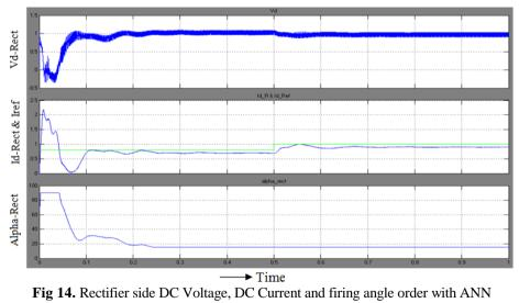
From the above graph  $I_{d\_R}$  and  $I_{d\_Ref}$  are compared to produce an error signal which gives the firing angle order  $(\alpha = 15.5 \text{ deg}).$
